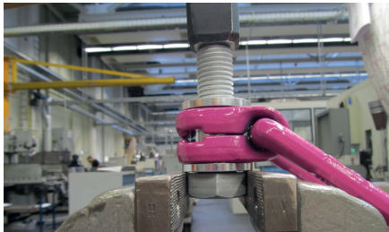
Pic. 6: Dismantling position of the ICE-LBG-SR
